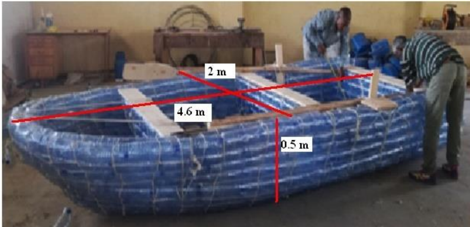
Fig.4: The boat that is made up of west plastic bottle
