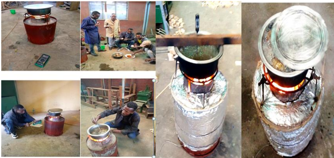
Fig 16: The pictures taken while the WBT and CCT experiments conducted
