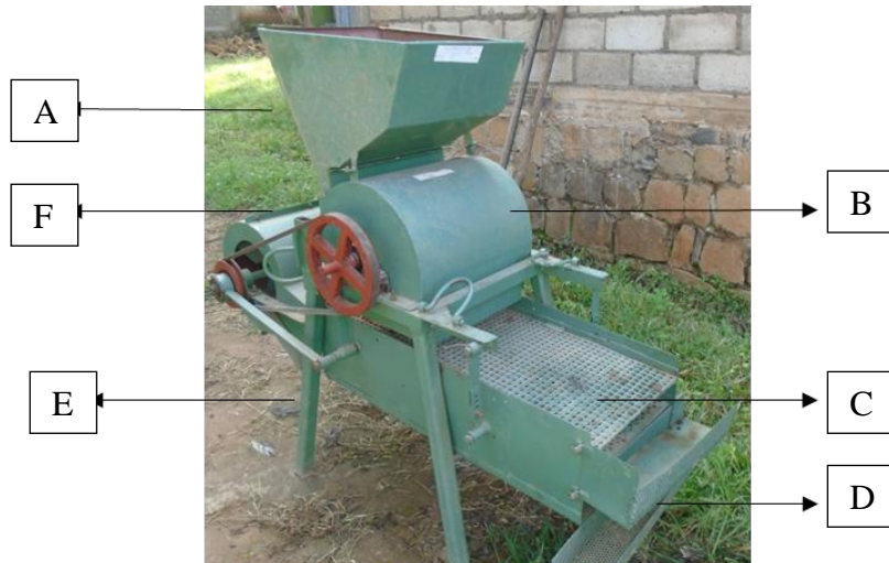
Figure 1. The pictorial representation of the sheller. A– Hopper, B– Drum unit, C– Sieve, D– Delivery unit, E– Frame, F– Fan
