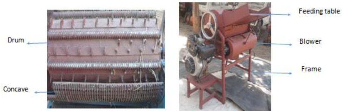
Figure 2. A prototype and its basic parts
