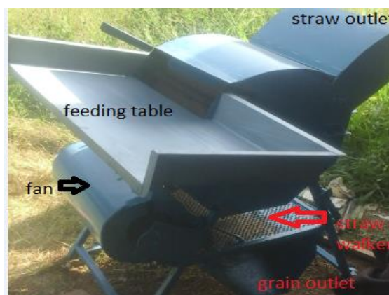
Figure 1. Description of rice threshing machine
