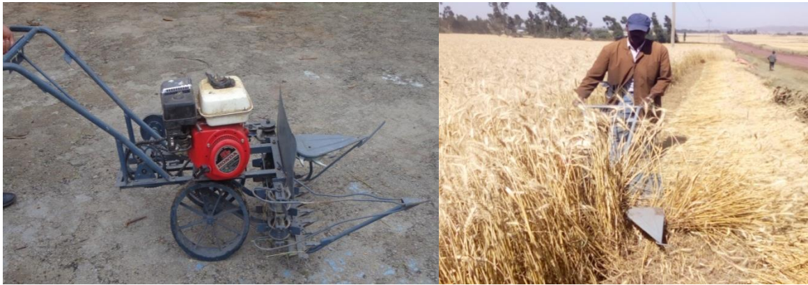
Figure 1. The developed engine operated reaper and during harvesting
