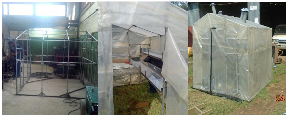
Figure 1. Prototype of polyhouse solar drier seems this when constructed
