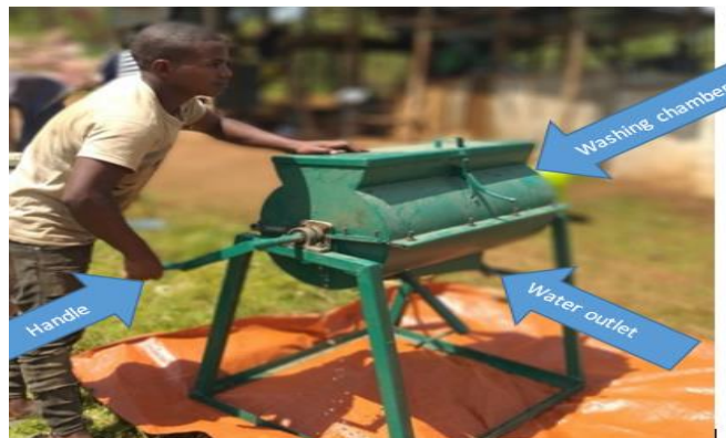
Figure 1: The developed manual operated coffee bean demucileger
