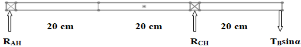
Figure3. Free body diagram of the main shaft on horizontal (XZ) plane
