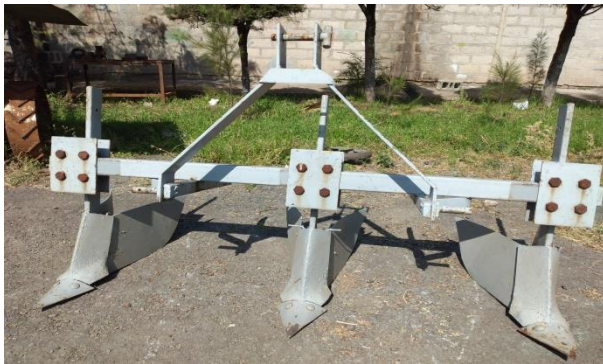
Fig.1. developed prototype of potato hiller
