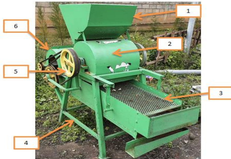
Figure2. The pictorial picture of the coffee de-huller (1.Hopper, 2.Drum, 3.Sieve, 4.Frame, 5.Pulley, 6.Fun)
